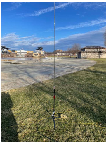
Antenna now on flat bar tripod with rock keeping it stable. It's extended the full 17ft 9". 40 M coil in place.
