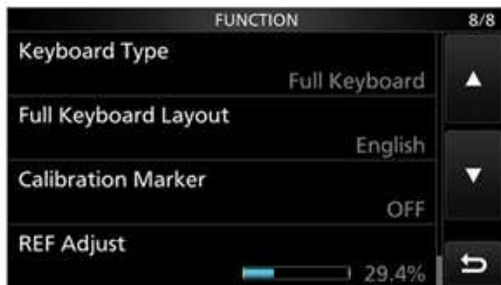
Figure 7 ICOM 7300 Reference Adjustment
